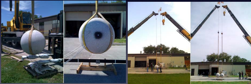
Figure 2. Granite spheres in equilibrium position. Left: Headache balls low near the spheres. Right: Headache balls moved higher up to minimize sphere wobble after impacts.
